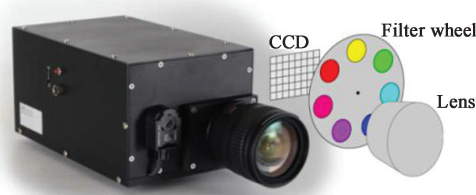
图5 七原色多光谱相机 [47] Fig.5 Multispectral camera using seven optical bandpass filters [47]
